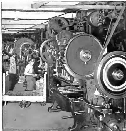
Stamping and forming presses in Simmons factory.
